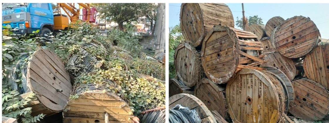
Cable lying in haphazard conditions at Barotiwala and at Parwanoo stores
